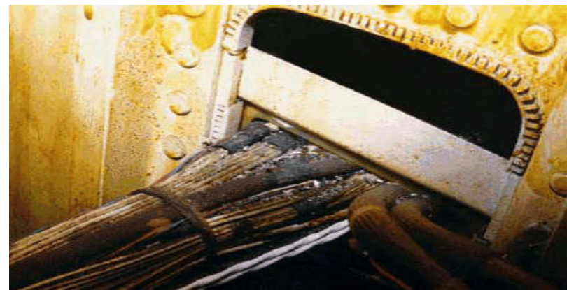
DRILL SHAVING AND CONTAMINATION ON WIRE BUNDLES
